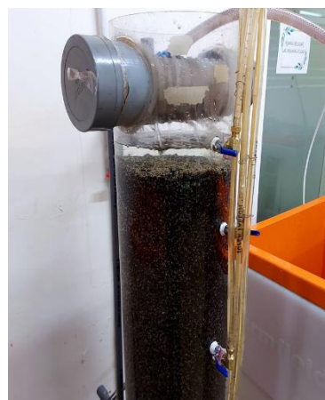
Figure 1. Laboratory Scale Filtration Reactor for Treating Raw Water PT. X
